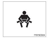
① This lamp lights ON for the first five seconds after starting the truck.
